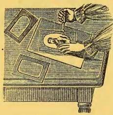
The accompanying cut represents the instrument in the act of trimming a photograph. It does not cut, but pinches off the waste paper, and leaves the print with a neatly beveled edge which facilitates the adherence of the print to the mount. Try one, and you will discard the knife and punch at once. For ovals and rounded corners it is worth its weight in gold.
